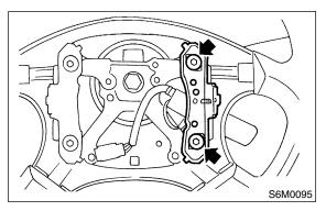
7) Disconnect horn and cruise control command switch connector, then remove cruise control command switch.
