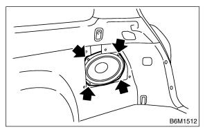
4) Disconnect harness connector, and then remove woofer.
