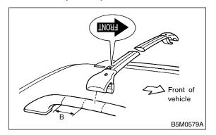
4) Tighten end support and lower clamp using TORX  $^{\!\!"}$  bolt T30.
