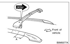
3) Set crossbar so that front direction arrow on the right top face of crossbar points in the direction of vehicle front, and place crossbar end support at position 152.4 mm (6.00 in) back from joint of rear roof rail support and roof rail.
