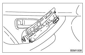
4) Remove three screws and clips.
