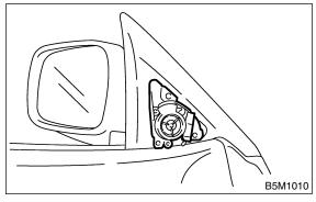
6) Remove seven clips of trim panel using clip remover to remove trim panel.
