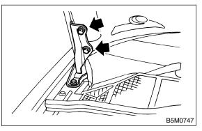
2) Adjust height at front end of hood. <Ref. to SL-40, ADJUSTMENT, Front Hood Lock Assembly.>
