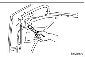
3) Remove bolts to disconnect hood from hinges.
