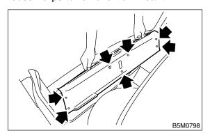
4) Remove hook (A) to pull off rear side of trunk side trim.
