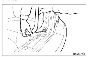
6) Loosen bolts to remove rear bumper.
