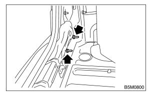
6) Loosen clips to remove upper beam (A) from bumper face.
