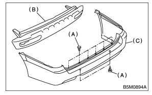
8) Remove resin beam from bumper beam.
