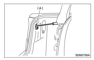
5) Remove two nuts from each side to remove rear bumper.
