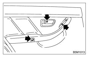
4) Remove seven clips of trim panel using clip remover to remove trim panel.
