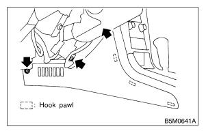
7) Remove passenger's airbag module. <Ref. to AB-14, Passenger's Airbag Module.>
