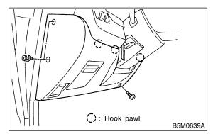
3) Remove lower column cover and disconnect harness connectors to steering column.
