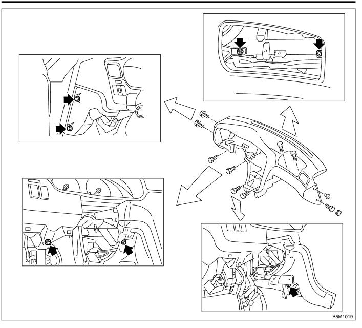
13) Disconnect harness connectors and remove instrument panel carefully.
