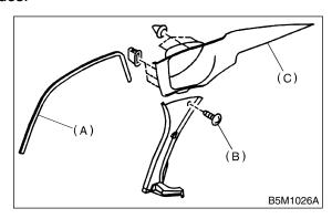
11) Remove clips, and then remove roof trim.
