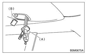
13) Remove clips and then remove roof trim.
