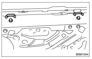
4) Operate power window switch to move glass as shown in the figure, and remove two nuts.
