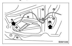
5) Loosen two screws to remove weatherstrip.
