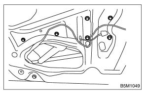
8) Loosen screws to remove motor assembly.
