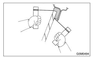
6) Pull the wire ends alternately to cut off the adhesive layer.
