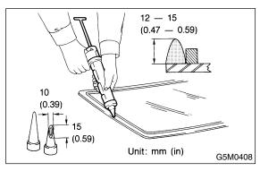
12) Apply adhesive to glass end surface as shown.
