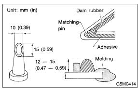
2) Install glass in the same procedure as for windshield glass. <Ref. to GW-24, INSTALLATION, Windshield Glass.>
