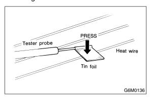
Measure voltage at wire center with DC voltmeter.
