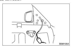
3) Loosen screws to remove mirror assembly.
