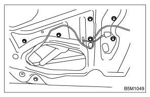
7) Loosen screws to remove motor assembly.
