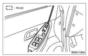
2) Disconnect electrical connectors from power window main switch and mirror switch.
