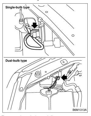
4) Remove three bolts and disconnect connectors, and then detach headlight assembly.
