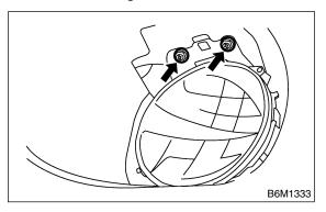
4) Remove two clips and lower the mudguard.
