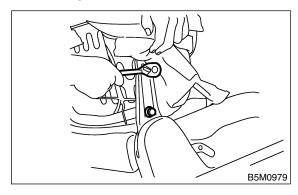
8) Remove hinge screw cover and screws, and remove seat back from hinge.
