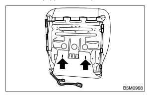
20) Remove hog rings. Tilt type vehicle:
