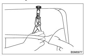
10) Remove hog ring on front face of seat.
