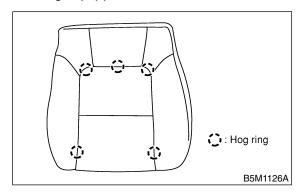
11) Remove hog rings, and then remove seat heater. (Seat heater equipped vehicle)
