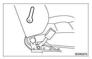
3) Remove hook at bottom, and then remove seat back board.
