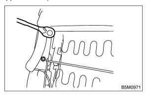
16) Remove the 4 bolts of seat hinge assembly, and then remove seat cushion.
