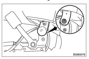
9) While picking up tip with a plier, remove headrest lock bushing.
