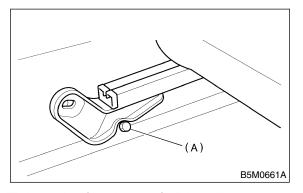
3) Tighten the four bolts of slide rail.
