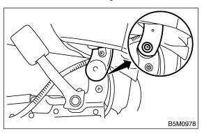
9) While picking up tip with a plier, remove headrest lock bushing.
