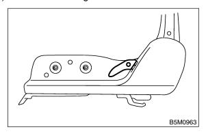
25) Remove hinge cover cap and screws.
