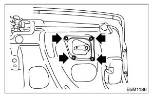
2) Remove the cable from trunk lid release handle.
