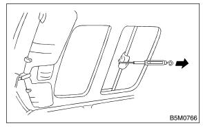
2) Pull spring scale to measure force required to move the sunshade.
