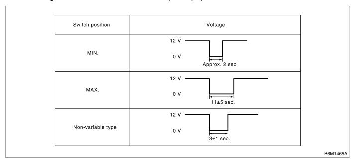
If operation is not as specified, replace the switch.
