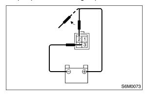
3) Connect battery and confirm that motor stops at automatic stop position after motor operates at low speed again.
