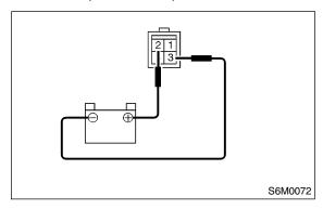
2) Connect battery to terminal of connector and remove terminal connections with motor rotated, and stop wiper motor through operation.
