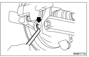
3) Suspend the disc brake assembly so that the hose is not stretched.
