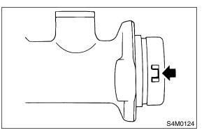
4) Using pliers, remove C-ring. (With VDC)
