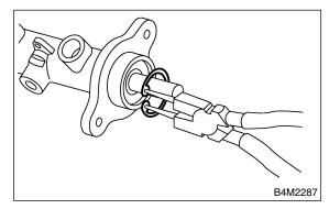
Extract primary piston assembly and secondary piston assembly.
