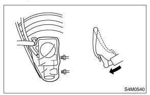
5) Close outlet plug with your finger, and release brake pedal.
