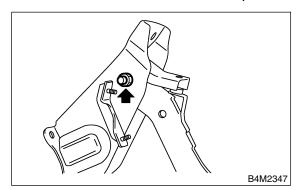
3) Remove bushing, spacer and spring.
