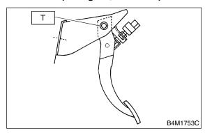
4) Set brake pedal position by adjusting position of stop light switch.
