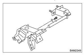
4) Remove bushing, spring and stopper.
