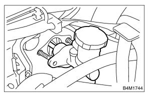
8) Remove bolts and nuts which secure brake and clutch pedals, and remove pedal assembly.
