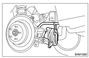
8) Remove disc rotor from hub.
