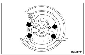
2) Tighten four bolts to back plate.
