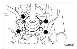
10) Remove hub unit bearing.
