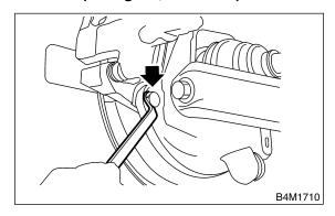
8) Install rear ABS sensor and brake cable bracket.
