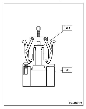
3) Using ST, press hub bolt out. ST 927080000 HUB STAND
