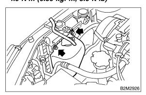
7) Install air intake duct.
