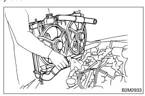
3) Install radiator brackets and tighten bolts.
