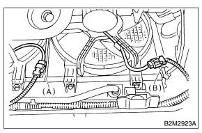
6) Disconnect radiator outlet hose from thermostat cover.
