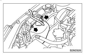
12) Disconnect radiator inlet hose from engine.
