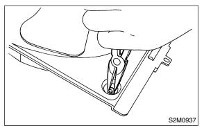
2) Remove nut which holds fan itself onto fan motor and shroud assembly.
