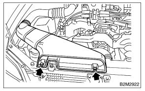
7) Remove bolts which hold sub fan shroud to radiator.
