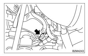
3) Disconnect rear oxygen sensor connector.
