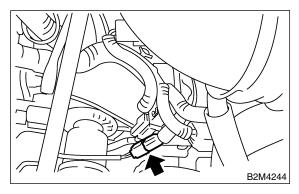
10) Connect front oxygen (A/F) sensor connector.
