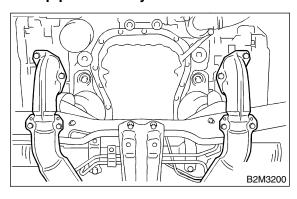
8) Remove bolt which installs front and center exhaust pipe assembly to hanger bracket.
