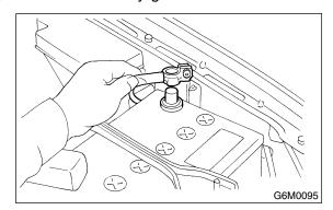
2) Disconnect front oxygen (A/F) sensor connector.
