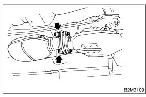
2) Separate rear exhaust pipe from muffler.
