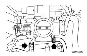
8) Remove bolts which install throttle body to intake manifold.
