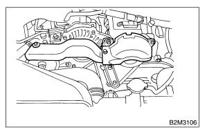
(3) Loosen lock bolt and slider bolt, and remove power steering pump drive V-belt.
