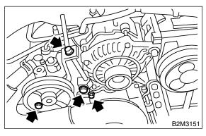
(4) Install power steering pipes onto right side intake manifold protector.
