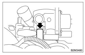
25) Install intake air temperature and pressure sensor.
