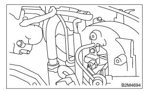
10) Disconnect engine coolant hose from throttle body.
