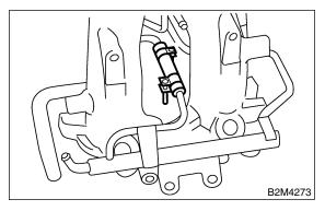
27) Loosen clamp which holds front right side fuel hose to injector pipe and remove the pipe from clamp.
