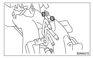
10) Tighten bolt which install injector pipe on intake manifold.
