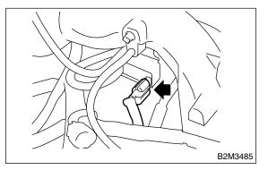
17) Disconnect air by-pass hose from purge control solenoid valve.
