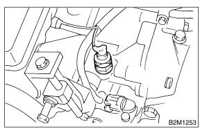
5) Connect connector to crankshaft position sensor.
