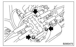
28) Connect connector to ignition coil and ignitor assembly.
