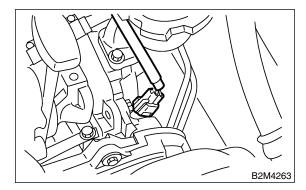
4) Connect connector to oil pressure switch.
