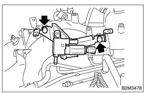
20) Connect air by-pass hoses to air assist solenoid valve.
