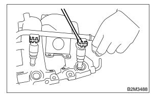
8) Tighten bolt which installs injector pipe on intake manifold.
