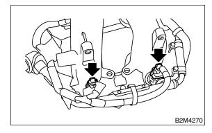
16) Disconnect connector from purge control solenoid valve.
