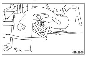
11) Install purge control solenoid valve.
