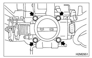
23) Connect connector to throttle position sensor and idle air control solenoid valve.
