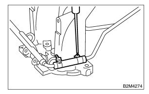
4) Install fuel injector pipe.
