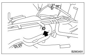
30) Remove fuel pipe assembly and pressure regulator, from intake manifold.
