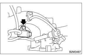
12) Connect hoses to purge control solenoid valve.
