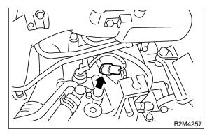
(3) Tighten bolts which install power steering pump on bracket.
