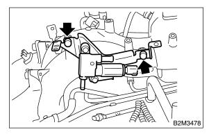
12) Disconnect pressure regulator vacuum hose from intake manifold.
