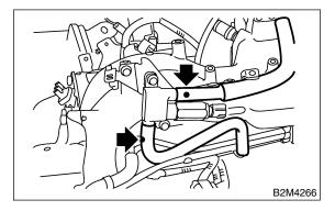
21) Connect connector to air assist solenoid valve.
