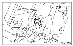
17) Disconnect connector from camshaft position sensor.
