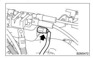
3) Remove ignition coil and ignitor assembly.
