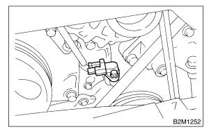
16) Disconnect connector from oil pressure switch.
