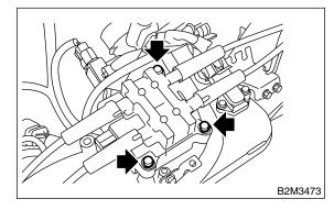
4) Disconnect connector from intake air temperature and pressure sensor.
