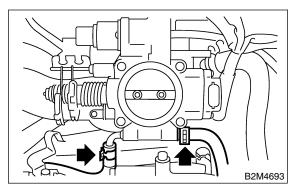
11) Connect PCV hose to intake manifold.
