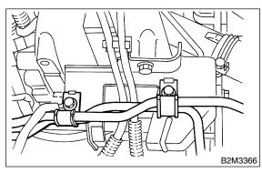
(5) Remove bolts which install power steering pump bracket.
