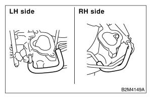
26) Loosen clamp which holds front left side fuel hose to injector pipe and remove the pipe from clamp.
