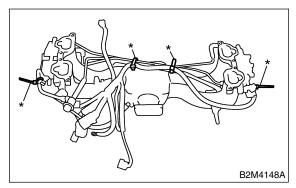
19) Remove engine harness from intake manifold.20) Remove purge control solenoid valve.
