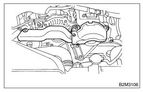
(8) Install resonator chamber.
