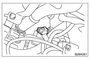
8) Install air cleaner case stay RH and engine harness bracket, and connect engine harness connectors to bulkhead connectors.
