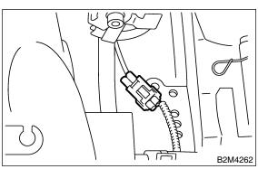
7) Connect connectors to engine coolant temperature sensor.
