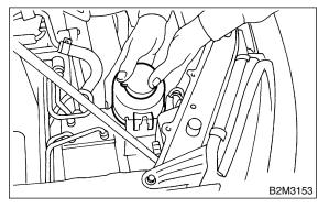
(8) Place power steering pump and tank on the right side wheel apron.
