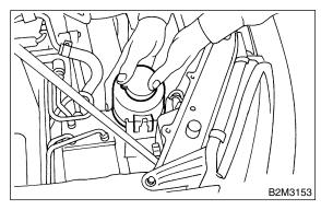
(2) Connect connector to power steering pump switch.
