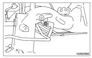
23) Remove two bolts which hold fuel pipes on the left side of intake manifold.
