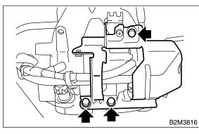
15) Disconnect connectors from fuel injectors.
