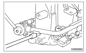
9) Tighten two bolts which install fuel pipes on the left side of intake manifold.
