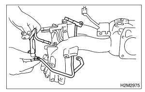
29) Remove bolt which installs fuel pipes on intake manifold.
