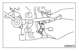
25) Disconnect air by-pass hoses from intake manifold.
