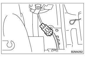
15) Disconnect connector from crankshaft position sensor.
