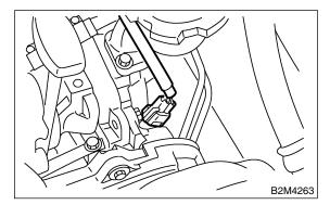
18) Disconnect fuel hoses from fuel pipes.
