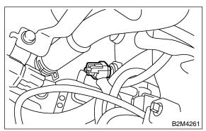
4) Remove engine coolant temperature sensor.
