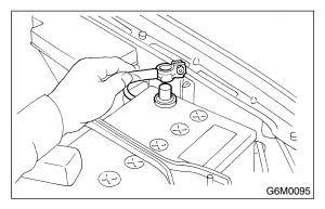
2) Remove bolt which installs crankshaft position sensor to cylinder block.
