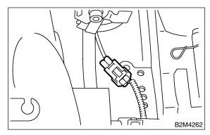
4) Remove knock sensor from cylinder block.
