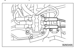
3) Disconnect connector from intake air temperature and pressure sensor.
