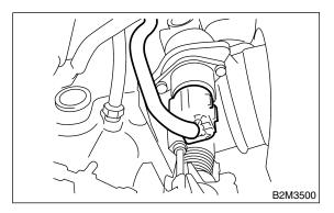
3) Remove idle air control solenoid valve from throttle body.
