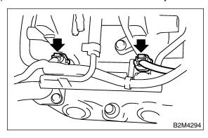
12) Remove bolt which holds injector pipe to intake manifold.
