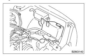
9) Remove spark plug cords from spark plugs (#2 and #4 cylinders).
