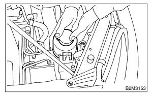
(7) Place power steering pump and tank on the right side wheel apron.
