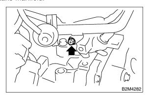
12) Remove fuel injector from intake manifold.
