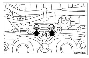
13) Remove bolt which installs injector pipe to intake manifold.
