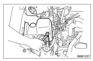
6) Remove spark plug cords from spark plugs (#1 and #3 cylinders).
