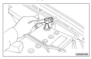
4) Remove two bolts which install washer tank on body.
