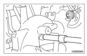
14) Remove bolt which holds fuel pipe on the left side intake manifold.
