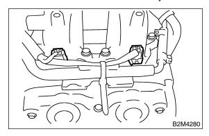
10) Remove bolts which hold injector pipe to intake manifold.
