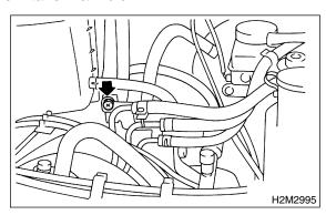
15) Remove fuel injector from intake manifold.(1) Remove fuel injector securing clip.
