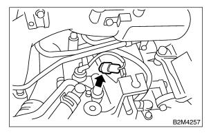
(6) Remove power steering tank from the bracket by pulling it upwards.
