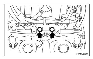
11) Remove bolt which install injector pipe to intake manifold.
