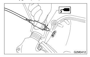
2) Install front oxygen (A/F) sensor.
