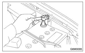
2) Remove lower cover. <Ref. to EI-37, REMOVAL, Instrument Panel Assembly.>3) Disconnect connector from fuel pump relay.
