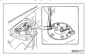
11) Remove bolts which install fuel sub level sensor on fuel tank.
