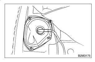
9) Disconnect connector from fuel sub level sensor.
