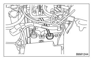
6) Remove spark plug with the spark plugs socket.
