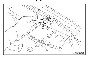
2) Disconnect washer motor connector.
