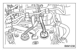
4) Remove spark plugs with the spark plug socket.
