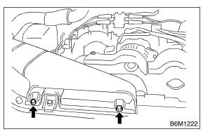
2) Remove bolt which installs air intake duct on body.
