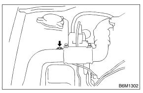
3) Remove air intake ducts as a unit.
