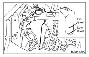
3) Attach radiator cap and reservoir tank cap properly.
