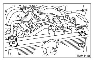
14) Detach power steering hose from the clip on the radiator.
