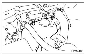
7) Install air intake duct.
