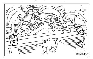
4) Attach power steering hose to the radiator.
