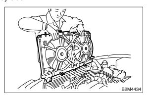
3) Install radiator brackets and tighten bolts.
