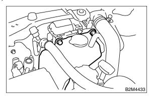
12) Disconnect radiator inlet hoses from radiator.
