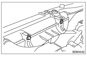
12) Remove radiator main fan motor assembly.
