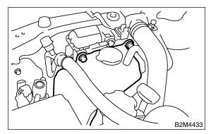
10) Disconnect radiator inlet hoses from radiator.
