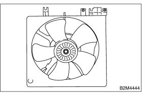
3) Remove screws which install fan motor onto shroud.
