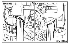
4) Install front exhaust pipe to rear exhaust pipe.
