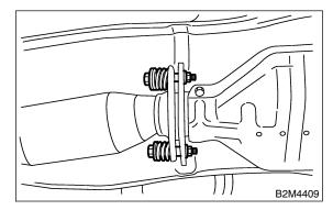
10) Remove bolts which hold front exhaust pipe onto cylinder heads.
