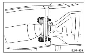
5) Tighten bolt which holds front exhaust pipes to hanger bracket.
