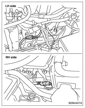
11) Install air cleaner case and air intake duct. <Ref. to IN(H6)-5, INSTALLATION, Air Cleaner.> and <Ref. to IN(H6)-7, INSTALLATION, Air Intake Duct.>
