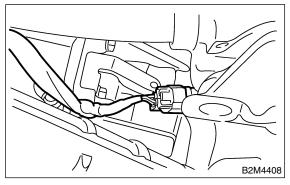
7) Install front oxygen A/F sensor harness to the clips attached to the cylinder head covers.
