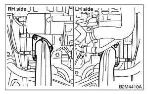
11) Remove front exhaust pipe from hanger bracket.
