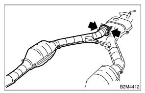
2) Install front exhaust pipe. And temporarily tighten bolt which installs front exhaust pipe to hanger bracket.
