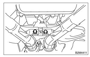
12) Separate front catalytic converter (RH) from front exhaust pipe.
